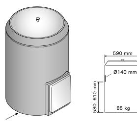
Adjustable legs (3 pcs): Lift the cauldron by about 50 mm and insert the adjustable leg's screw end in the hole in the plastic part. Put the cauldron back on its surface and adjust the legs to ensure that it is level.
